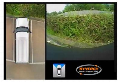
**Default View on start-up**: The 360° 'Bird's eye' view provides the driver with a complete view of the vehicle surroundings, offering assistance when parking or manoeuvring in restricted spaces. The system automatically switches view when the car is placed in reverse gear, or when the turn indicators are used.
