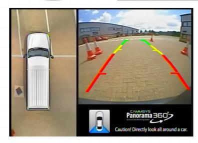
**Reversing**: Smart Vision is especially useful when reversing into or out of parking spaces, as it offers the driver the top view combined with a wide angle rear view, to negotiate even the tightest of spaces. If required the driver can switch to a full screen view of the front or rear cameras using the control switch.
